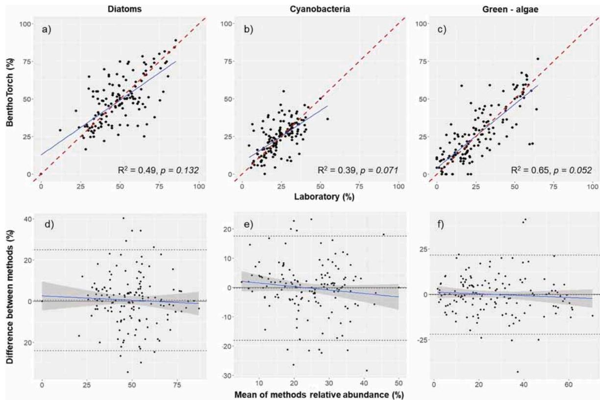
Fig. 5. Biovolume proportions (%) of diatoms (a, d), cyanobacteria (b, e), and green algae (c, f) measured with BenthosTorch (*in situ*) and laboratory (standard) methods on natural substrates ( $n = 144$ ). Top panels show regression lines (blue) with respect to the equality line (red). Bottom panels show the bias between method agreement (black) with 95% confidence intervals (dotted lines) and regression lines (blue).
