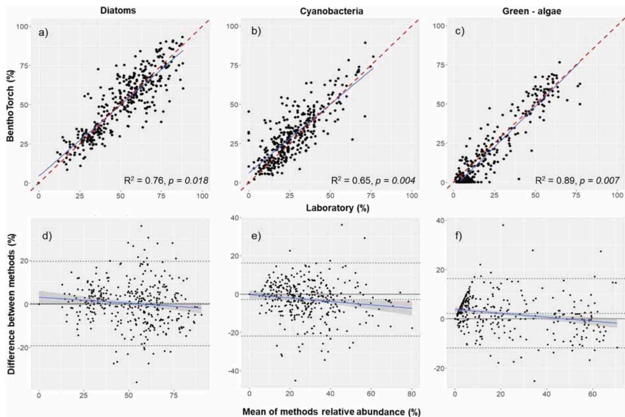
Fig. 4. Biovolume proportions (%) of diatoms (a, d), cyanobacteria (b, e), and green algae (c, f) measured with BenthosTorch (*in situ*) and laboratory (standard) methods on artificial substrates ( $n = 359$ ). Top panels show regression lines (blue) with respect to the equality line (red). Bottom panels show the bias between method agreement (black) with 95% confidence intervals (dotted lines) and regression lines (blue).
