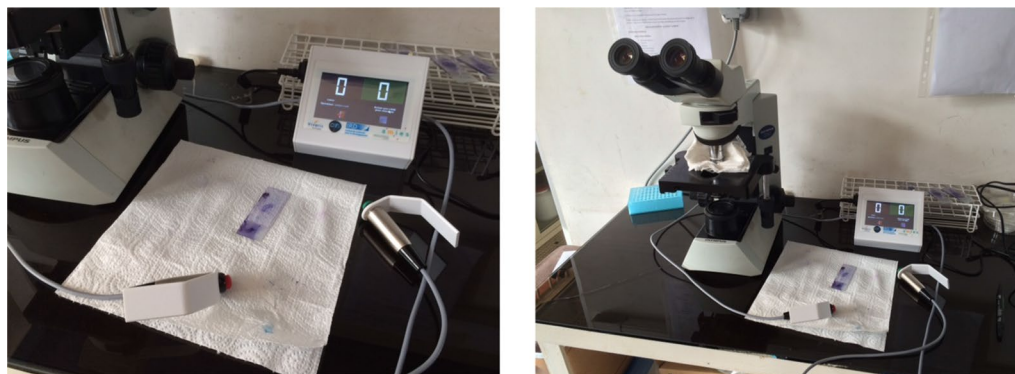
Fig. 1 The timed tally counter. The left counter (Red button) counts the parasites and the right counter (Green button) counts the leucocytes. The current number of the two counts is displayed with the corresponding color on the LCD screen (here: 0 and 0 for the two buttons)
