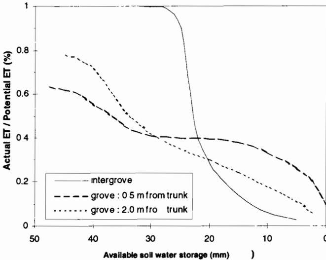
Figure 5.1. Soil water extraction in banded vegetation. Alice Springs (Australia). (Modified from Slatyer 1961.)
