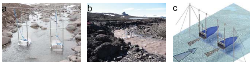
Figure 4. River Bedload Traps (RBT) in (a) Fosa Creek and (b) Siodło Creek (modified from Szilo and Bialik [46]); (c) schematic diagram for the bedload transport technique (Kociuba [56]).
