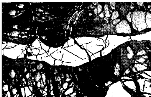
Fig. 5. Vein-like area of millerite with an inner area of pentlandite. X 25
