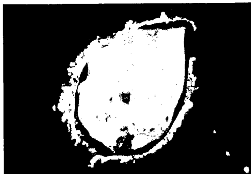
Fig. 3. Magnetite surrounded by pentlandite which the magnetite appears to have nucleated. X 30
