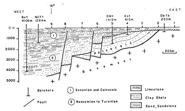
Fig. 3. Interpretative geological model through the southern part of the S-M basin along the MT line.
