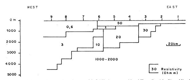
Fig. 2. Geoelectrical cross-section across the southern part of the S-M basin, constructed from MT soundings (after Ritz and Vassal, 1986).
