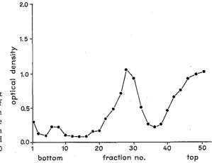
Fig. 1. Sucrose density gradient centrifugations of GCV. 2 ml of virus preparation was layered on a gradient of 5-40% sucrose (26 ml total) in 0.05 M sodium phosphate buffer, pH 7.5, and centrifuged for 2 h at 25,000 rev/min in the SW 25.1 rotor
