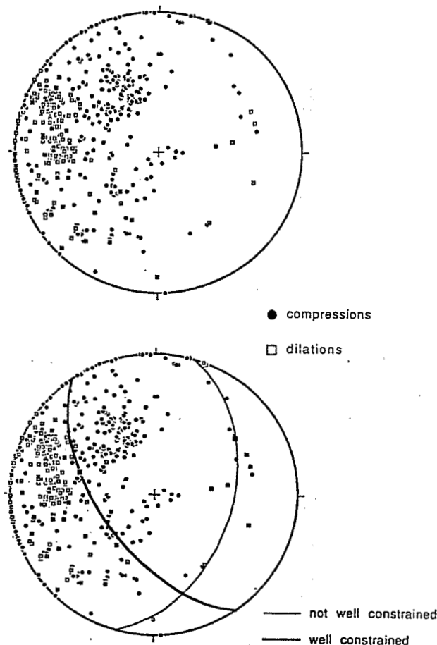
Fig. 10. Composite focal mechanism of the October-November 1986 swarm using the four stations on Efate and all earthquakes during the swarm with depth less than 30 km. The bottom figure shows a possible solution.
