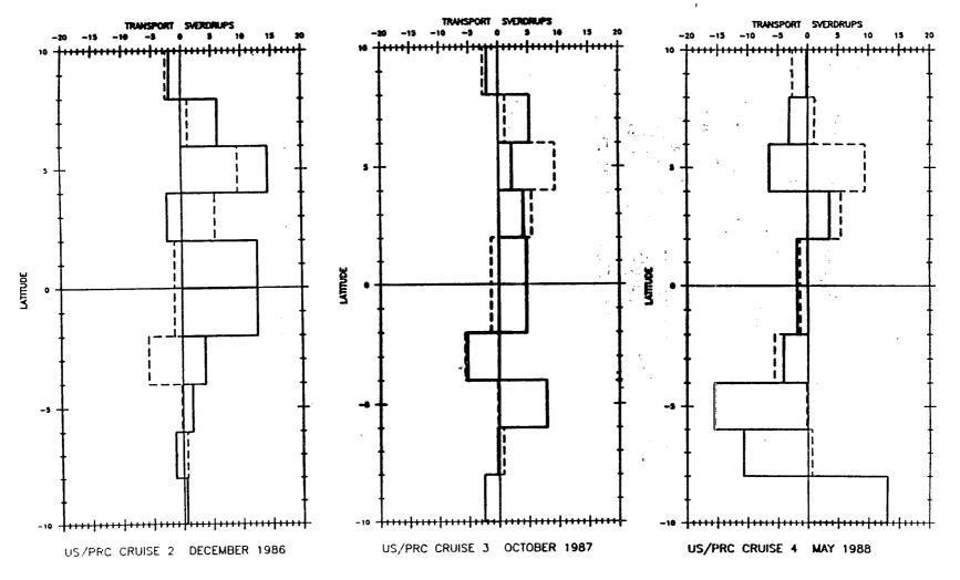
Fig.4. Meridional distribution of zonal geostrophic transport of water above the 23.5 kg m  $^{-1}$  sur  $^{-1}$  sec. The dashed line gives the annual mean transport
