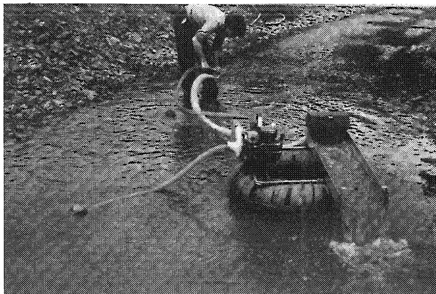
Fig. 3. Portable suction dredge used to collect a preconcentrate of heavy minerals in the field
