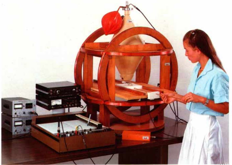
Sample study using a SQUID magnetometer (developed by D. LETI).
