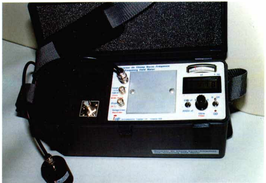
Flux-meter for measuring low frequency magnetic fields. Manufactured under licence by the companies ARPE and ICAP (developed by D. LETI).
