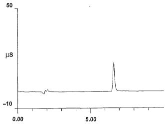
Fig. 2. Elution profile of phytic acid standard. Separation of phytic acid on an Omnipac Pax-100 column; eluents: 200 mM NaOH, Water-Isopropanol (1:1, v/v) and Water (18 m $\Omega$ ); detection: chemically suppressed conductivity using and ASRS-I 4 mm).
