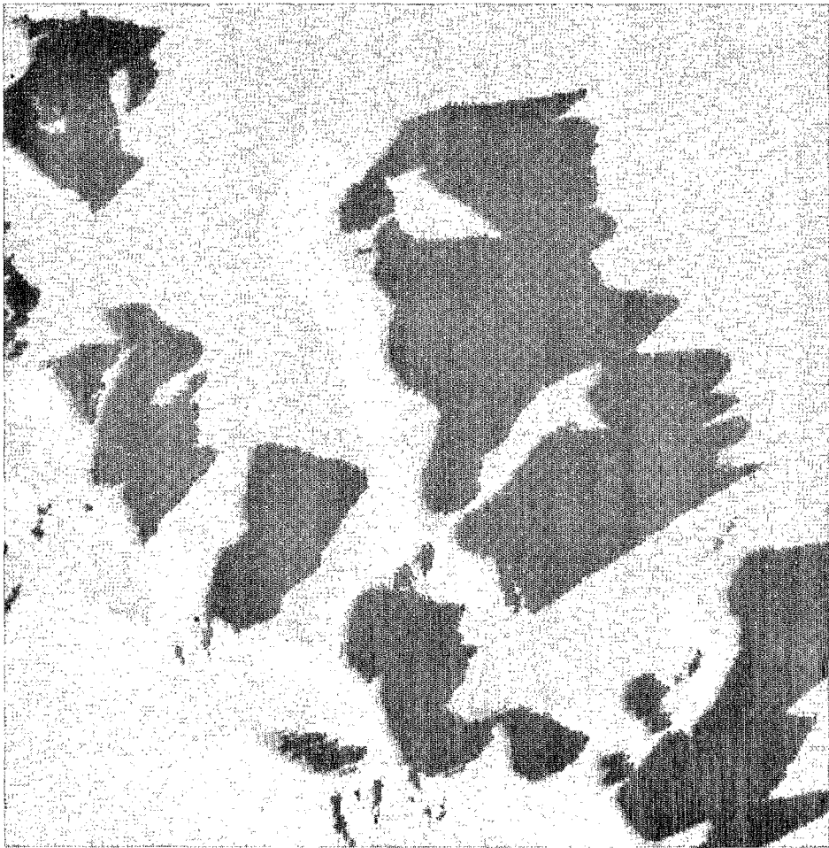
Figure 4. Shadow distribution calculated from the DTM for a Sun azimuth and elevation corresponding to the available SPOT image.
